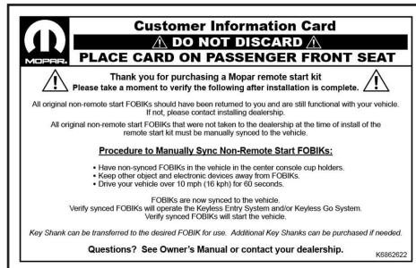
**IMPORTANT:** After installing this kit, all the non-remote start FOBIKs which came equipped with this vehicle will still be functional and can be used as intended except to perform remote start function. This applies to both Admin and KeySense type FOBIKs. **DO NOT DISCARD ORIGINAL FOBIKs AFTER INSTALLATION IS COMPLETE.** **RETURN ALL FOBIKs TO CUSTOMER.**
